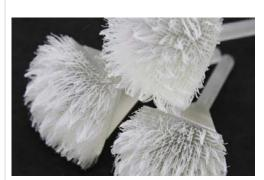
Researchers at MIT's Media Lab have recently developed a way to print hair-like structures using 3D printing technology. This will pave the way to design passive actuators and swipe sensors. In Addition read more about this technology in their MIT's Media Lab report.
